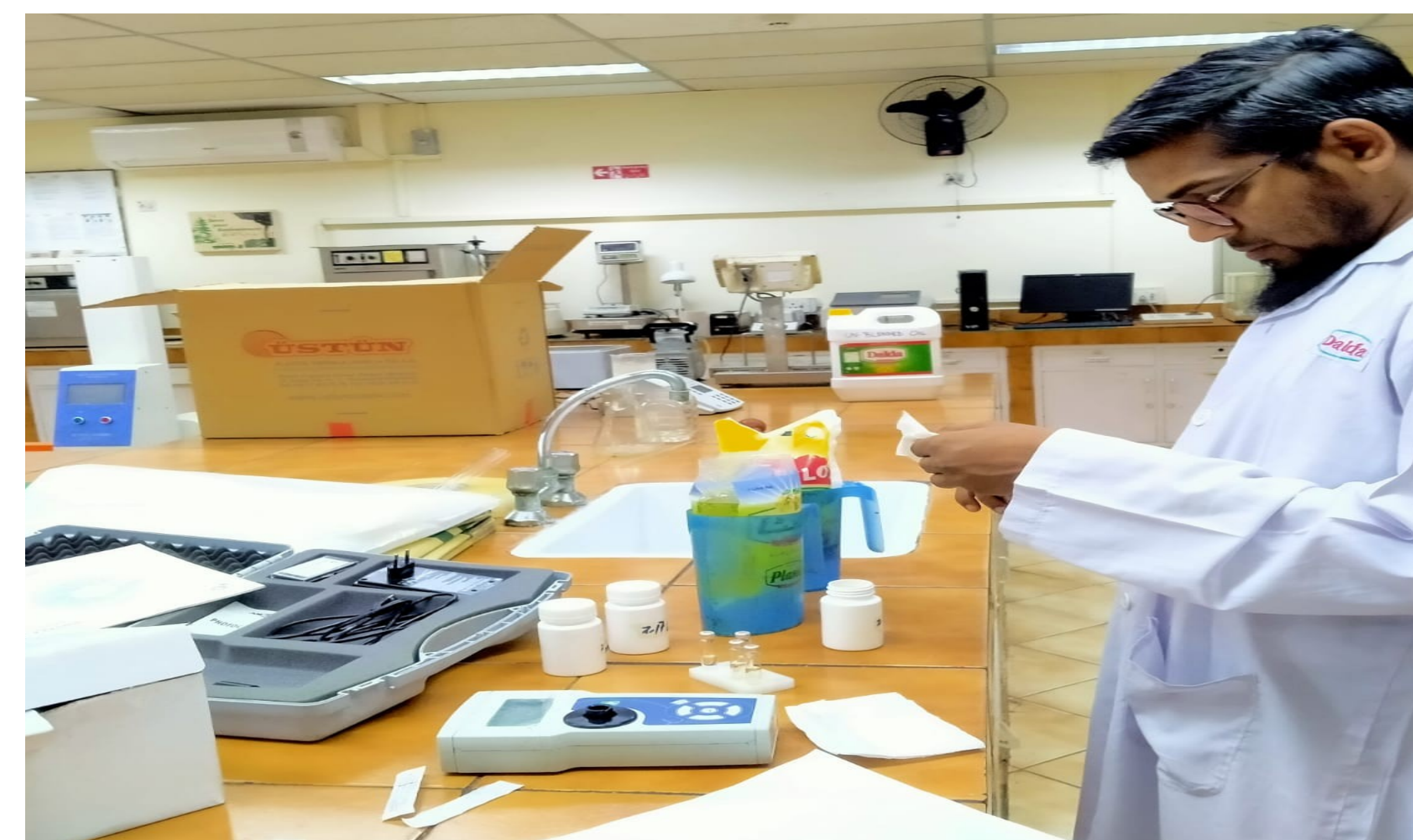
Figure 2: Quality Assurance test being performed for Vitamin A in edible oil using iCheck Chroma 3 at a local edible oil mill in Karachi, Pakistan
