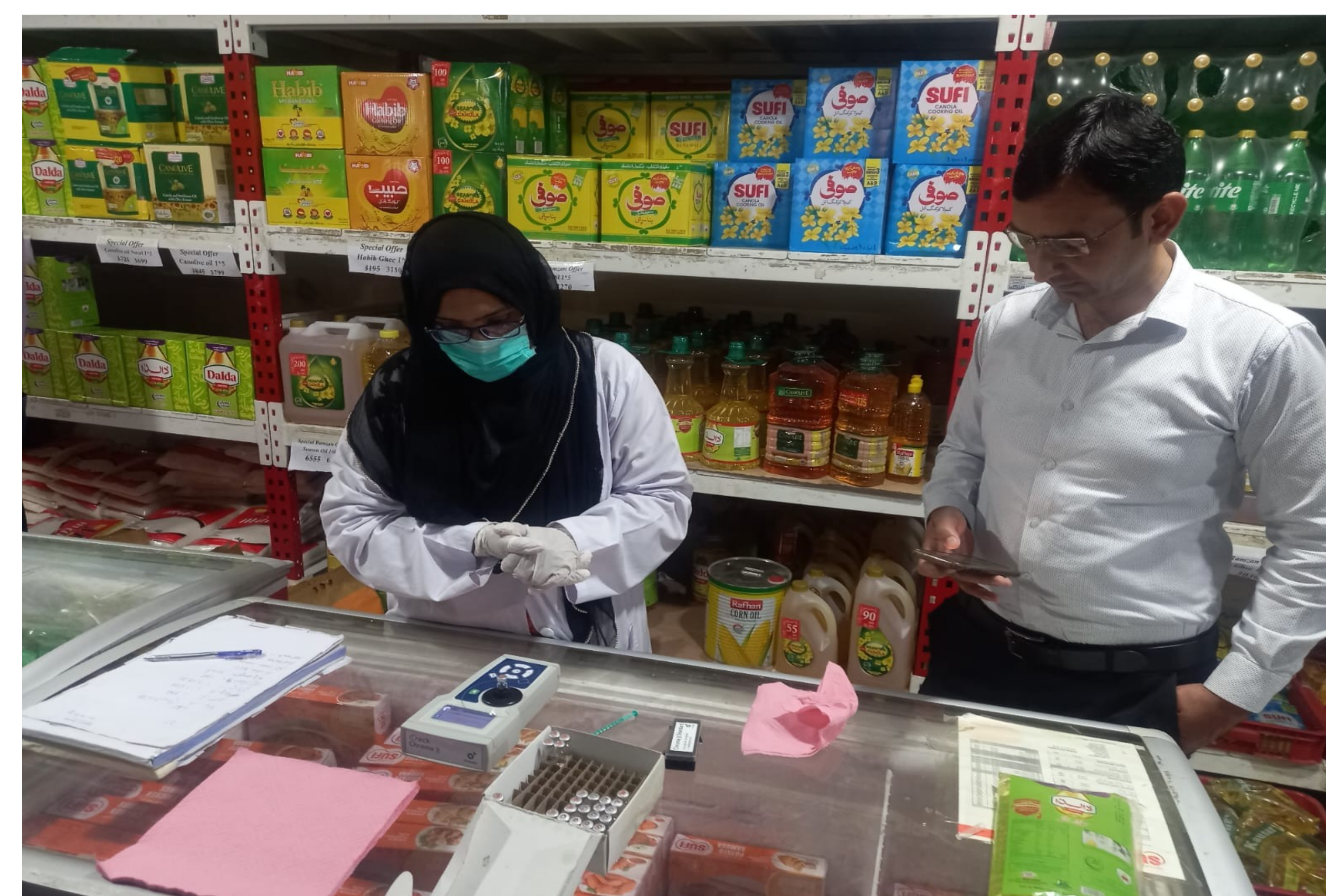
Figure 3: Punjab Food Authority official testing the level of vitamin A in edible oil using iCheck Chroma 3 device during a market visit in Gujranwala, Punjab, Pakistan
